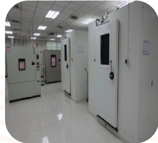
Thermal Cycle Test -45°C to +85°C Damp Heat Test 85°C, 85% RH
